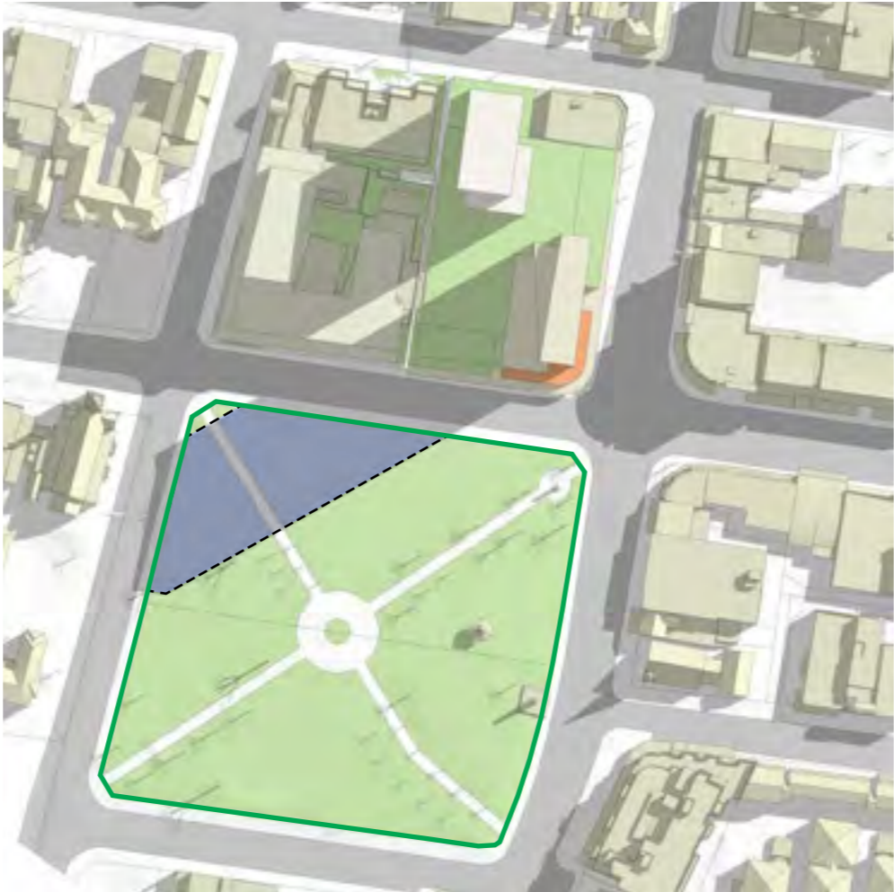
16% of Prince Alfred Square in Shadow 10am Daylight Savings Time (9am Solar Time)
